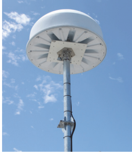
^ TCI 641 antenna in radome
